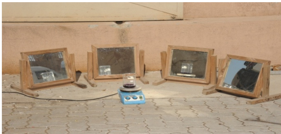
Figure 2. Photocatalytic degradation of direct sky blue5B dye experimental set up.
